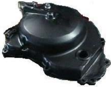
Figure 3.1: Modified clutch cover
