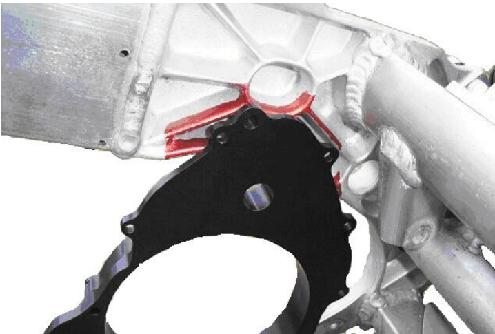
Figure 3.2: Frame to be cut out for clutch cover clearance
